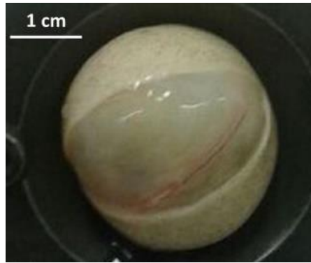
Figure 1: Bulge inflation test from a previous study showing layer delamination before complete failure.
