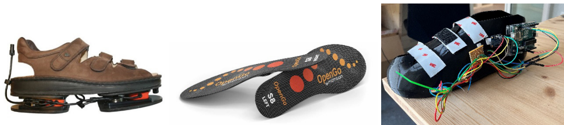
Figure 1: Left. Instrumented outsole with forces and moments sensors. Middle. Instrumented insole. Right. Developed instrumented shoes.
