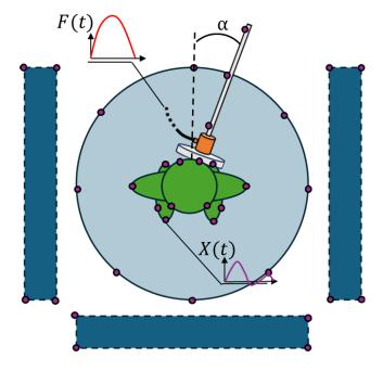
Left hand side: Picture of the experimental setup used in (Chatagnon et al., 2023). Right hand side: A very sophisticated way to push people against walls with an instrumented pusher.The setup is similar to (Chatagnon et al., 2023), with the addition of walls being placed at a controlled distance of the subject. Purple dots are motion capture markers and the orange cylinder represents the force sensor.
