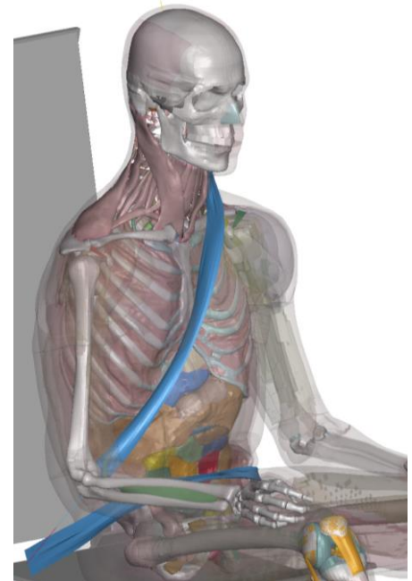
Fig. 1. Example of HBM simulation with a GHBMC detailed model ( www.ghbmc.com ). With 2.5M elements and most anatomical structures, the model better describes the human response than dummies but is also much more computationally intensive. It can be morphed and positioned to describe the diversity of occupants.
